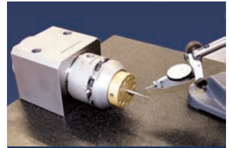
Presetting with Presetting Spindle and Adjustable Clamping Element
