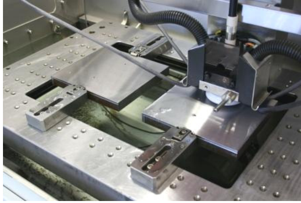
Workpieces fixation by means of 4 rulers WZ150L
