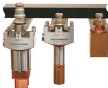
Storing with different clamping journals (H 6.611, H 5.511 and MINIFIXplus HCU5...)
